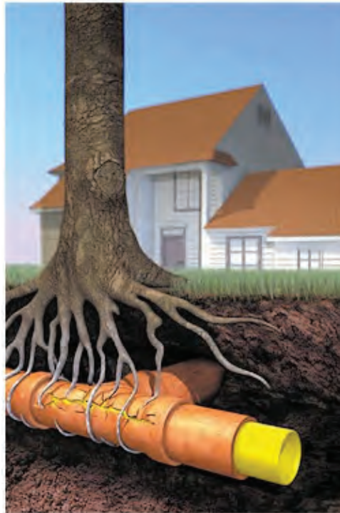
Figure 15: Avoid planting trees and shrubs above or near leach fields or plumbing lines.
